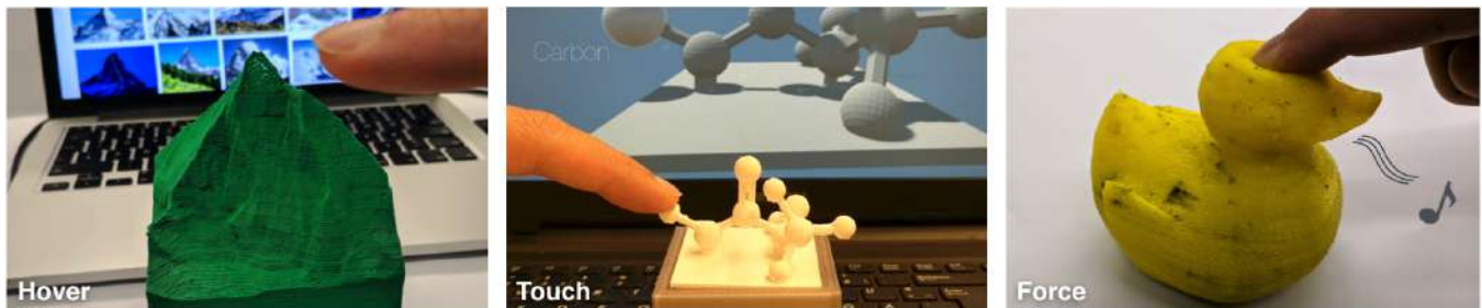
Figure 1: Trilaterate is a fabrication pipeline that enables users to 3D print hover-, touch-, and force-sensitive objects.
