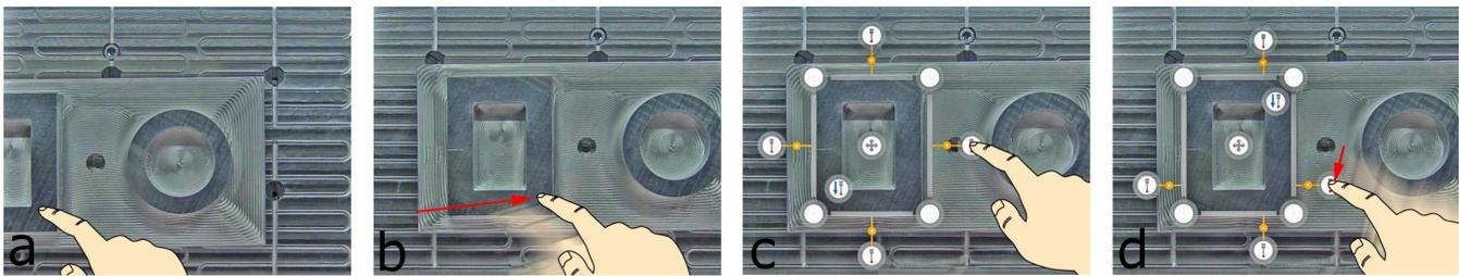
**Figure 1:** CaMea supports users in the process of initializing a workpiece in a CNC milling machine. We mounted a camera inside the machine and allow the user to move (a,b) the camera through touch gestures to align the camera with the workpiece. Once aligned, the user can select (c) and move (d) the touch points for the probing tip on screen.
