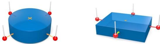
**Figure 2: Typical probing points for different geometries of workpieces. From left to right: (1) circle, outside and (2) square, outside**
