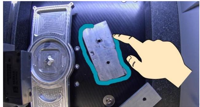
**Figure 5: CaMea allows users to draw the outlines of a workpiece roughly onto the camera image. We use a template matching algorithm to extract the type of the shape.**
