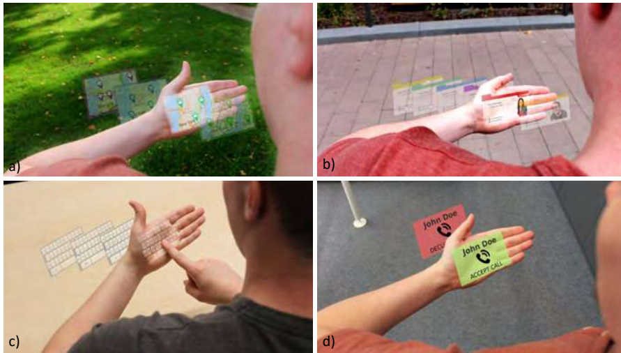
Figure 3.15: Example usecases for proximity-based interaction with HMDs. Proximity-based interaction can be used to browse through different views and visualizations of a data set (a) or to scroll through a list of items (b). Additional touch input can be used to interact with different visualizations (c). Further, shortcuts can be used to perform actions by raising the arm at certain distances from the body (d).
