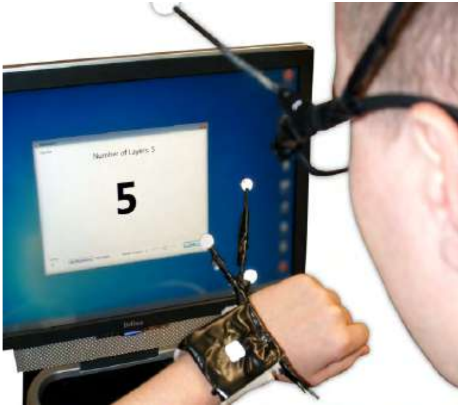
Figure 3.8: The setup of the controlled experiment with two retro-reflective apparatuses mounted on the participant's head and wrist, and the display showing the current task.
