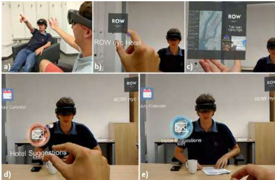
Figure 4.3: The interaction techniques of CloudBits: Users can (b) grab&move information drops freely in the space. To access information, users can grab an information bit and (c) open the hand with the palm facing upwards. Private information drops can (d,e) be shared with other users through grabbing and moving them towards another user. The color encodes if they are public or private.
