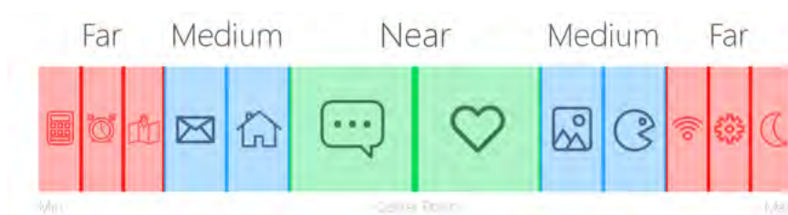
Figure 3.14: Design Guideline: Focus on the Convenient Range Use the near and medium layers for frequent and common interactions, use the far layers for irreversible interactions.
