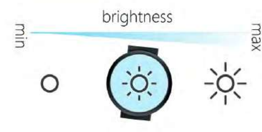
Figure 3.17: Example application for continuous interaction: A brightness control that lets the user modify the value by moving the arm alongside the line of sight.
