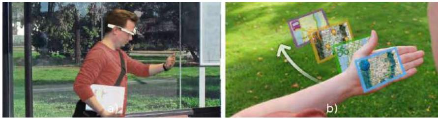
Figure 3.2: A map application as an example of one-handed (a) proximity-based interaction with a linear layered information space. The user can browse map layers by moving his hand through the space (b).
