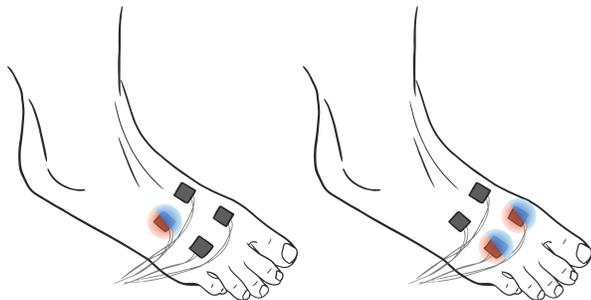
(a) *ThermoFeet* attached to the foot. With one or two Peltier elements activated with either a WARM or COOL stimulus.
