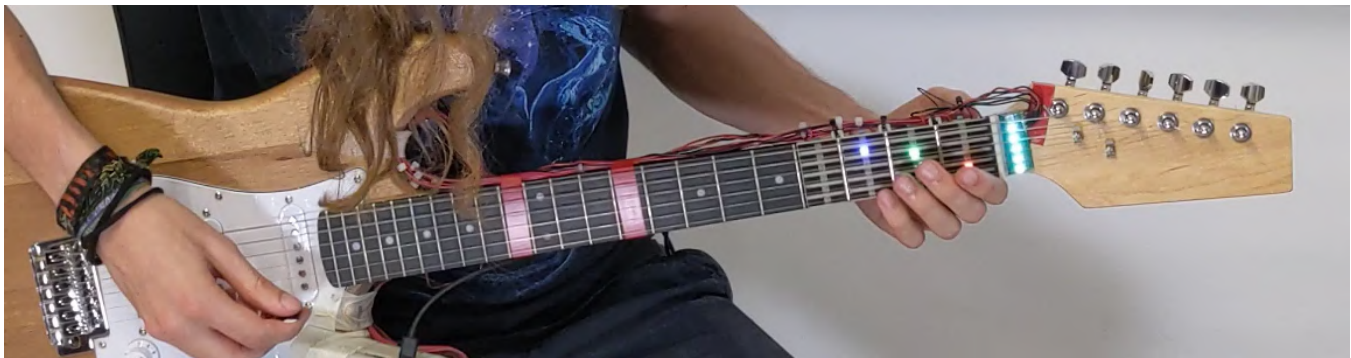
Figure 1: We present Let's Frets , a modular guitar learning concept with three feedback modules: (1) visual indicators, (2) finger position capturing, and (3) a combination of both modules.
