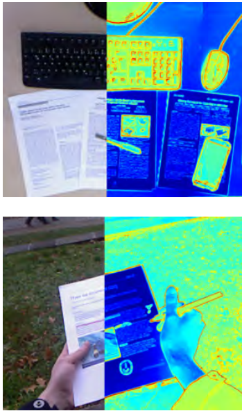
Figure 1: Colorized projectability map (dark blue=good projectability, red=bad projectability) of a conventional office desk (top) and a mobile paperwork scenario (bottom)
